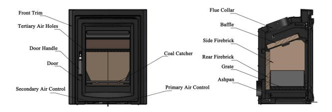
Fig 2 – Stove Assembly and controls
