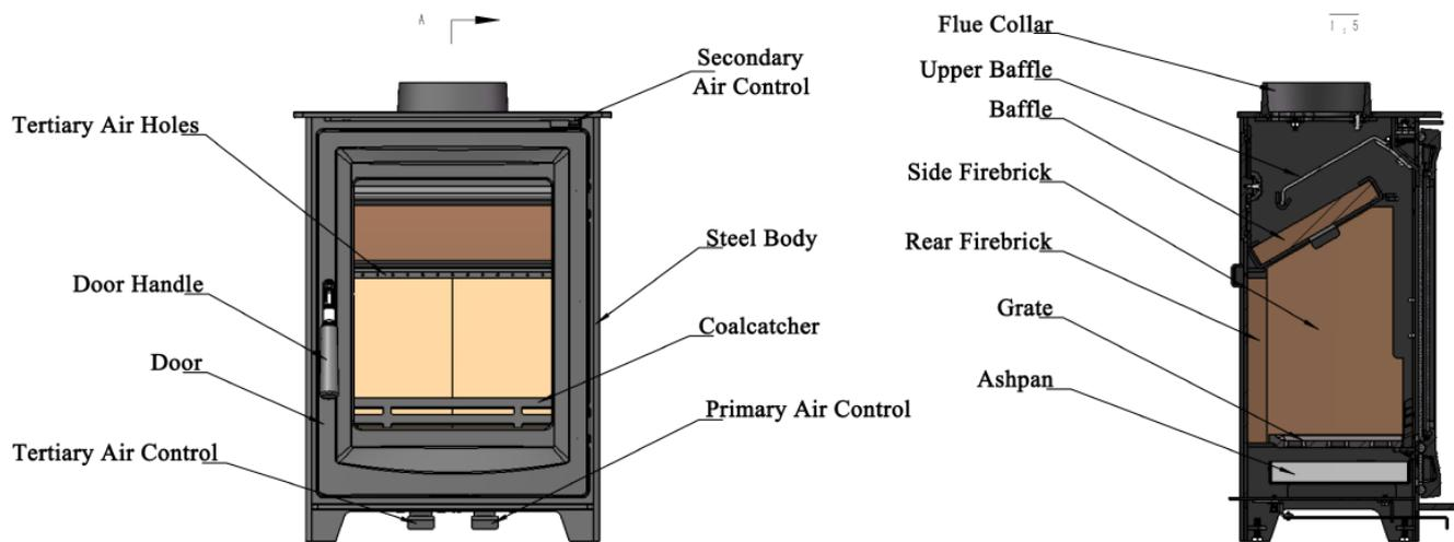
**Fig 2 – Stove Assembly and controls**
